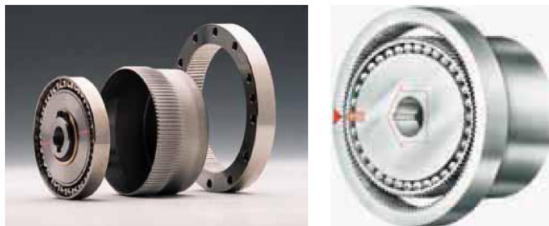
Figure 6.19: The harmonic drive. The rotation of the elliptical wave generator meshes the teeth of the flexspline and circular spline resulting in low backlash and high torque transmission. (Courtesy of HD Systems, www.hdsi.net .)
