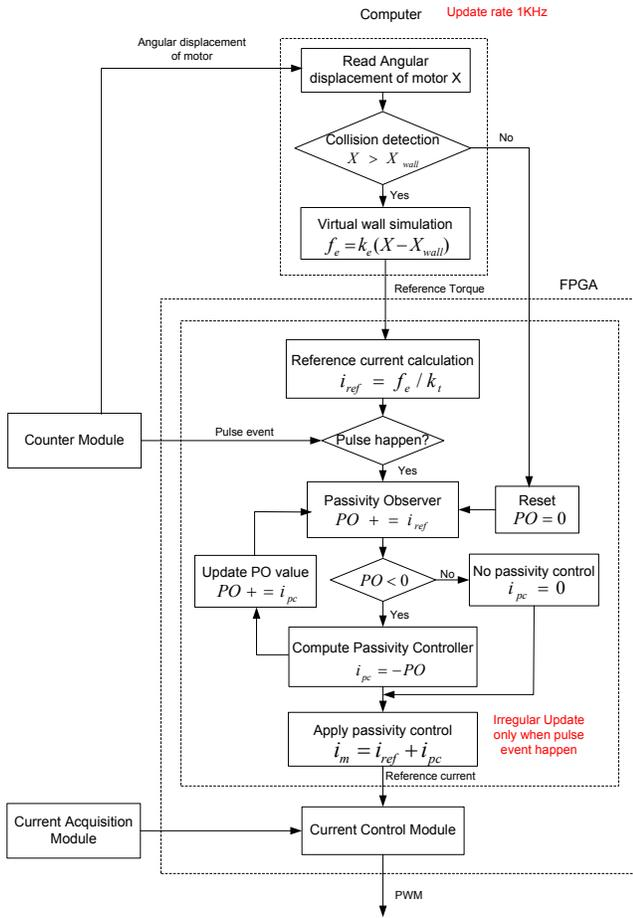
Fig. 4. Flow chart of PO/PC algorithm
