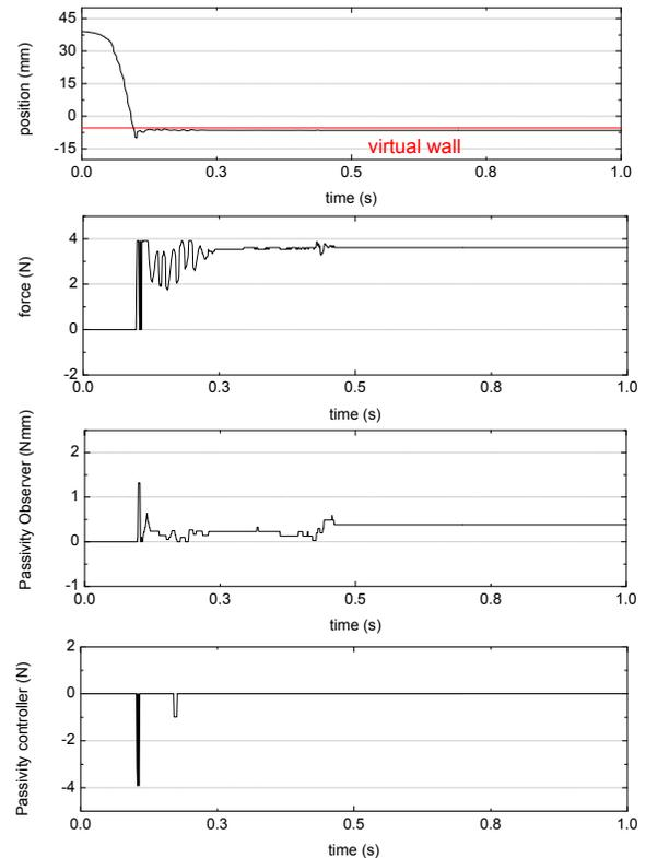
Fig. 9. Experimental results for the case when the FPGA based PC was activated. Interaction was stable, noise behavior was removed.
