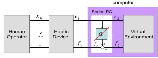
Fig. 1. Conventional PO/PC for one-port network with impedance causality
