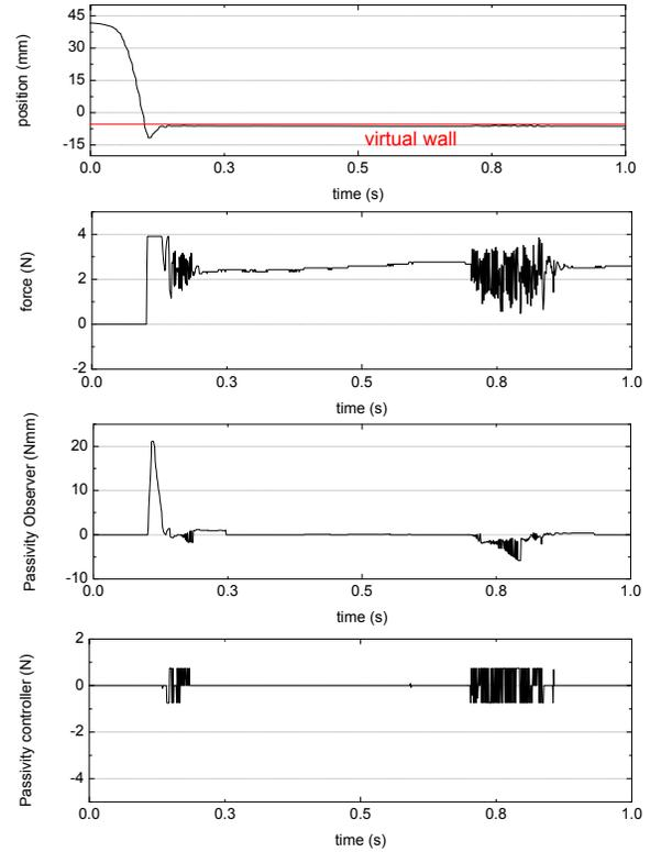
Fig. 8. Experimental results for the case when the conventional software based PC is turned on. Interaction was stable, but characterized by noise behavior.
