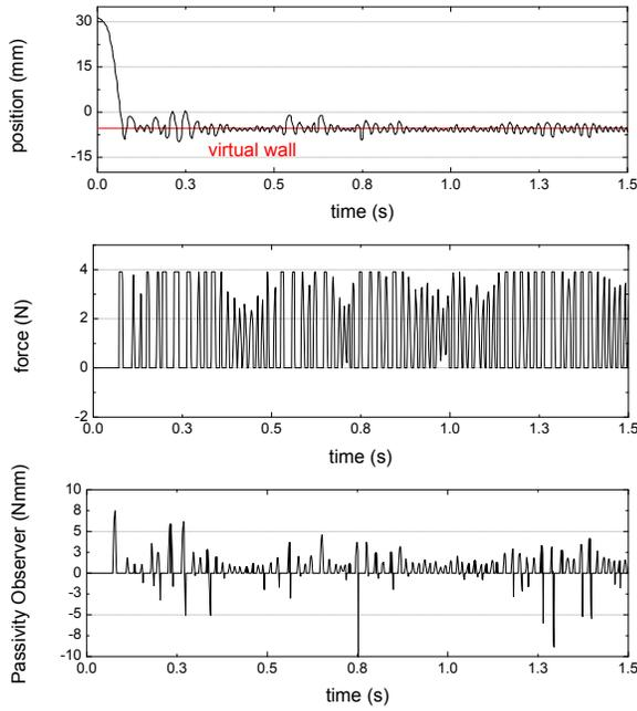
Fig. 7. Experimental results for the case when PC was not activated. Interaction was unstable
