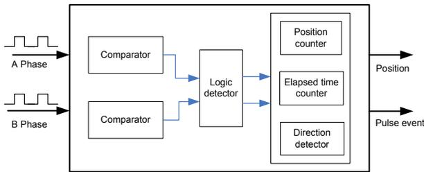
Fig. 3. Block diagram of encoder counter
