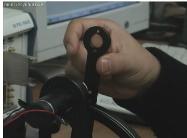
Fig. 6. Human operator pushes the device to contact with the virtual wall
