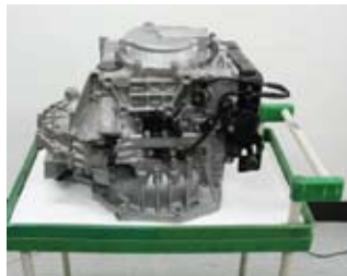
Fig. 2 Automatic transmission from Hyundai Sonata.
