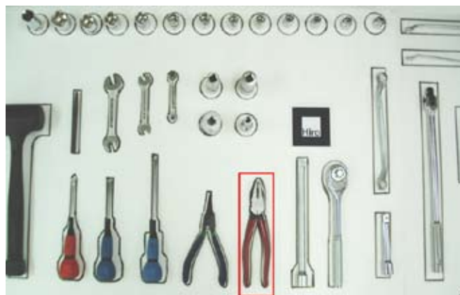
Fig. 7 Indicating required tool with the help of augmented reality.
