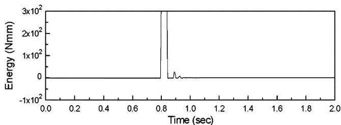
Fig. 8. Actual energy behavior with the new PO/PC approach for high-stiffness VE  $K = 120$  kN·m.
