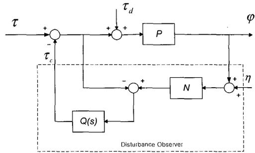
Fig. 3 Disturbance observer based control scheme of the ROV.
