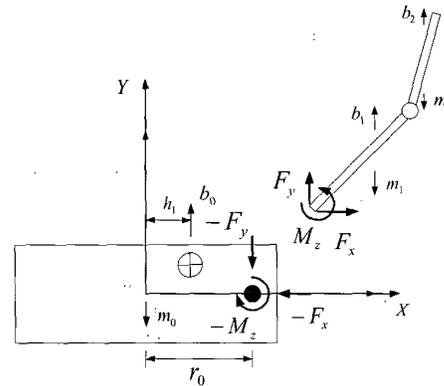
Fig. 1 Interaction forces between the ROV and the manipulator.
