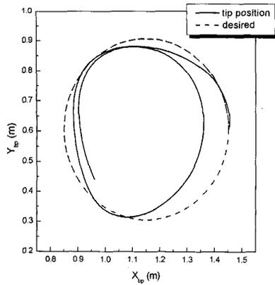
Fig. 5 Trajectory tracking performance of the end-effector without the base F/T sensor and the disturbance observer (DO).
