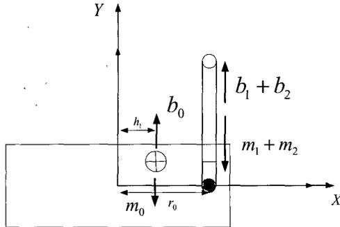
Fig. 2 Equilibrium posture of the vehicle/manipulator system.
