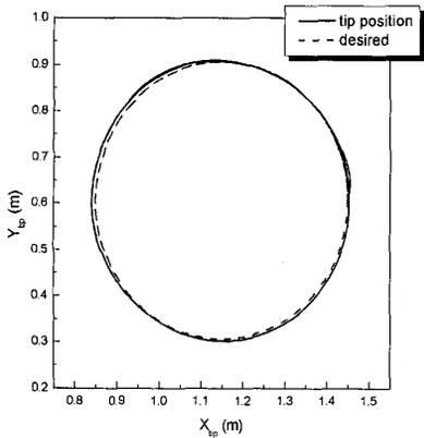
Fig. 7 Trajectory tracking performance of the end-effector with the base F/T sensor.
