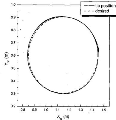
Fig. 9 Trajectory tracking performance of the end-effector with the DO.
