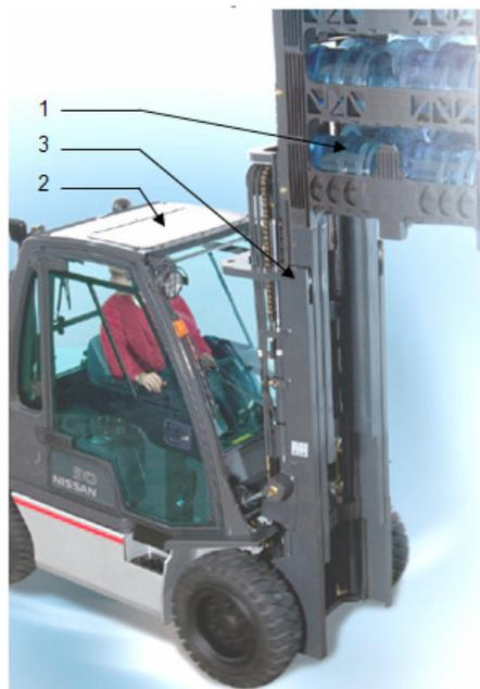
Fig. 1 Driver’s view is significantly reduced by the loads 2, the mast configuration 1, and the rugged overhead guard 3.
