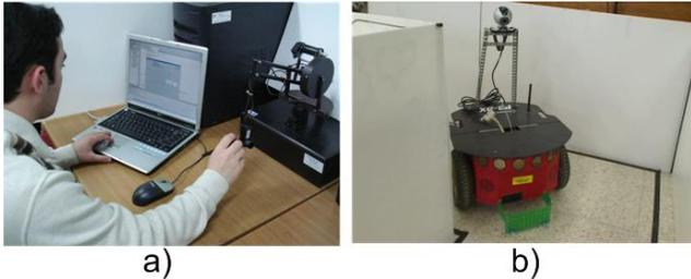
Figure 4: Human-operator and master setup during simulation and experiments (a) and the mobile robot during teleoperated by human-operator (b)
