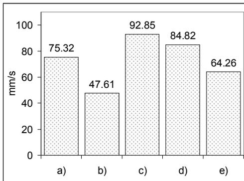
Fig. 8. Average speed of the mobile robot in teleoperation with different command strategies: a) position-speed strategy; b) position-position strategy; c) hybrid strategy with manual switching; d) hybrid strategy with manual-automatic switching; e) hybrid strategy with automatic switch.
