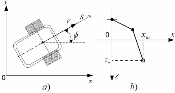
Fig. 1. Configurations of the master manipulator and the mobile robot.
