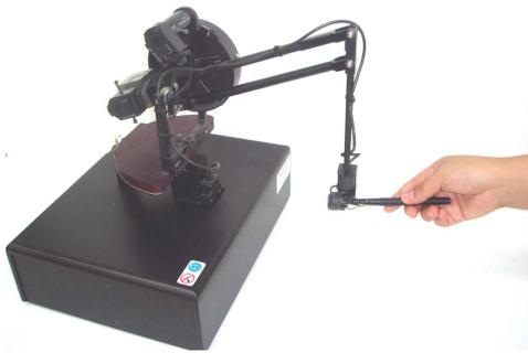
Fig. 2. Haptic device Phantom Premium 1.5A from SensAble Technologies, Inc.
