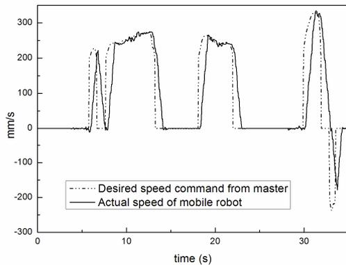
Fig. 5. Desired speed command from master device and actual speed of mobile robot graphs.
