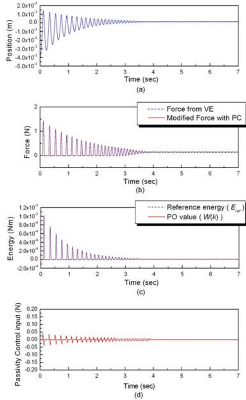
Fig. 10. Contact response with the PC force holding and the energy ignoring method as well
