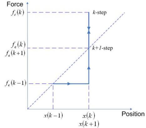
Fig. 4. Position vs. force response when the velocity become zero after the PC action
