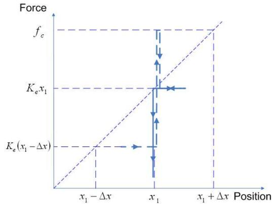
Fig. 7. Actual position vs. force response when the sign of the velocity is changed during low velocity
