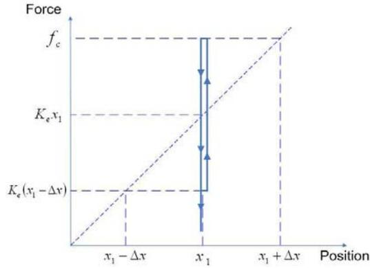
Fig. 6. Actual position vs. force response when the sign of the velocity is suddenly changed in one sample time
