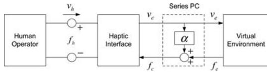
Fig. 1. Haptic interface system with series type PC for simulation
