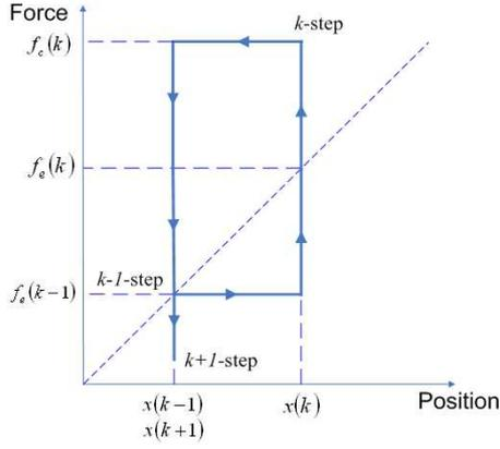
Fig. 3. Position vs. force response when the velocity sign is changed in one sample time
