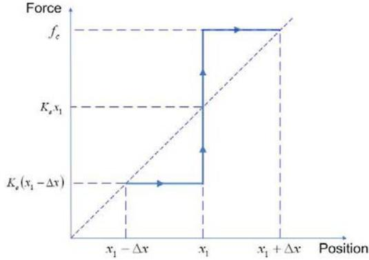
Fig. 9. Actual position vs. force response when the PC force is held while the velocity is zero
