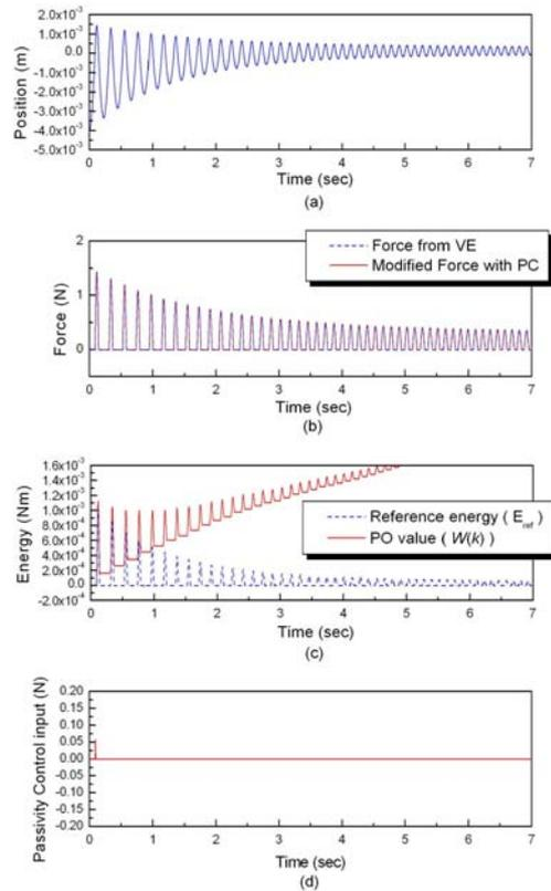
Fig. 5. Contact response with the energy following PO/PC, based on filtered velocity, for the high stiffness VE ( $K = 1000N/m$ ). The PO value was greater than the reference energy value even though the contact was unstable.
