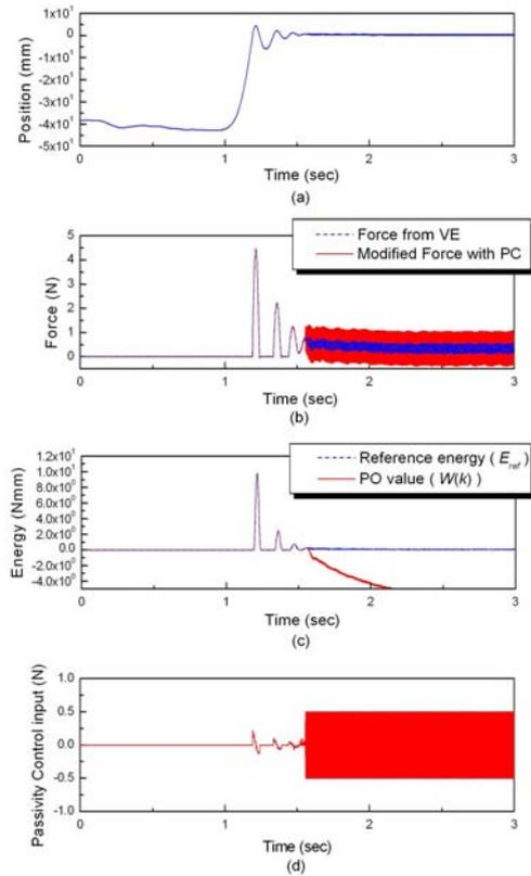
Fig. 11. Experimental result with the PO/PC without the proposed methods
