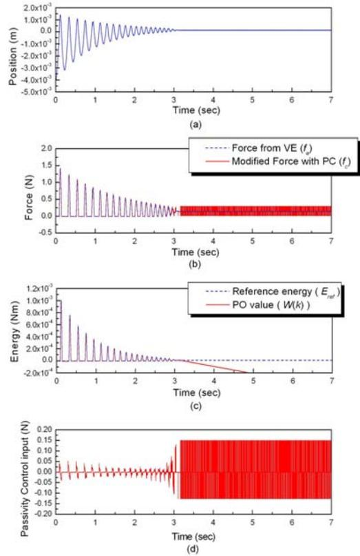
Fig. 2. Contact response with the energy following PO/PC [16] for the high stiffness VE ( $K = 1000N/m$ ). PC was noisy during the period of low velocity
