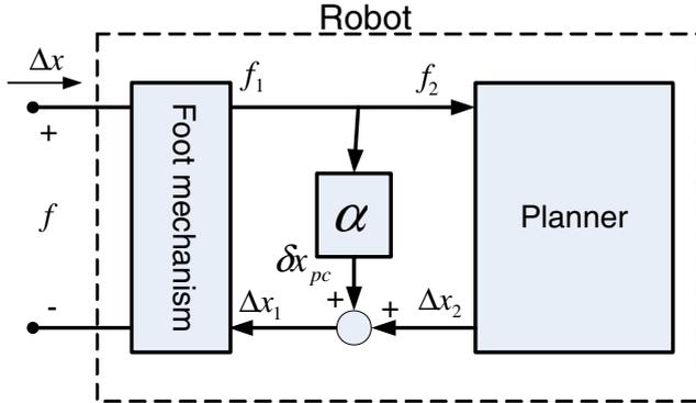
Fig. 4. One-port network with PO/PC.
