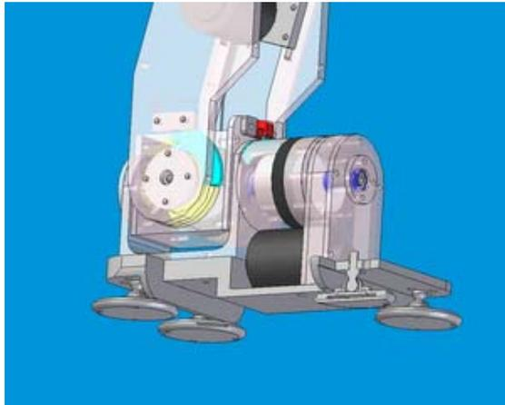
(a) Foot structure with four FSRs.
