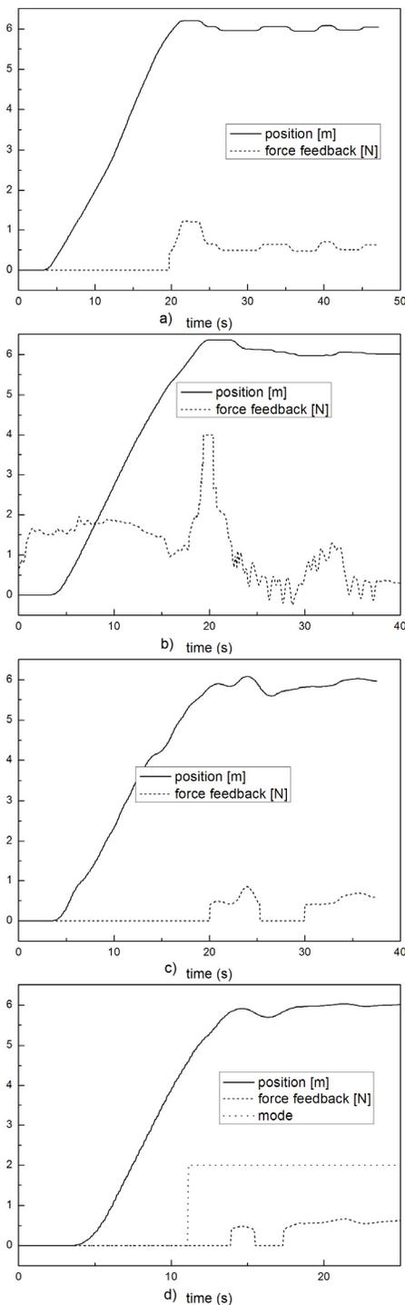
Fig. 8. Experimental results for mobile robot positioning, when textual information and force feedback is provided to human-operator. (a, b) position-speed, (c) position-position and (d) hybrid control strategies.
