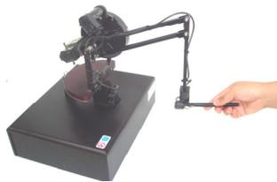
Fig. 3. Haptic device Phantom Premium 1.5A from SensAble Technologies, Inc.
