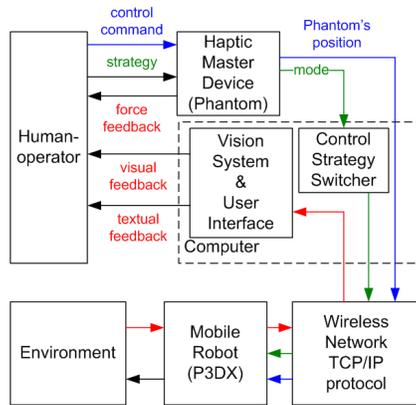
Fig. 2. Architecture of the experimental setup.
