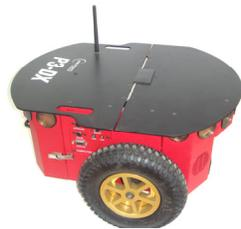
Fig. 4. Mobile robot Pioneer 3-DX from MobileRobots, Inc.
