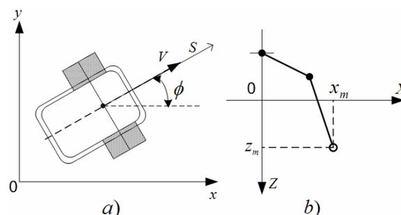
Fig. 1. Configurations of a two-wheeled mobile robot (a) and a master device (b).
