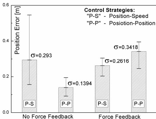
Fig. 9. Position error diagram for different control strategies with and without force feedback.
